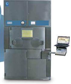
Specifically designed to accomplish the latest GMP guidelines for the preparation of gamma and beta radiopharmaceuticals, the NMC PRI is a GMP grade A hot cell, with a GMP grade B pre-chambers. Equipped with a Laminar Air Flow on the total working surface and inflatable seals. Its large inner room and specific equipment make the NMC PRI a remarkably flexible working instrument for many applications.
